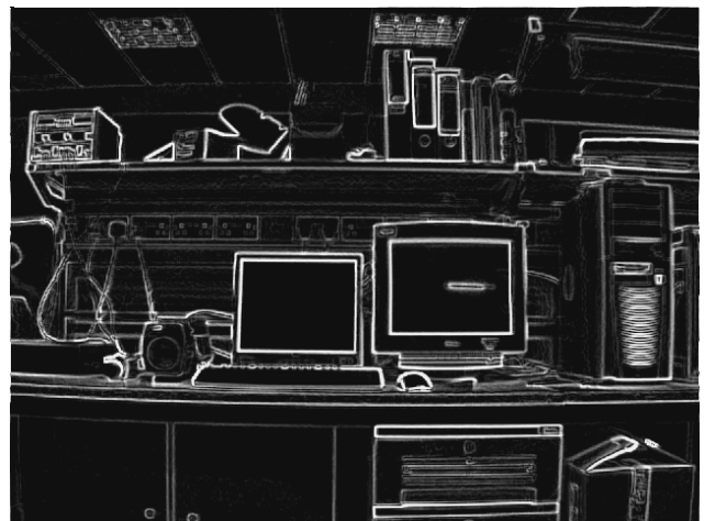
Figure 4 Video Image After Edge Detection
