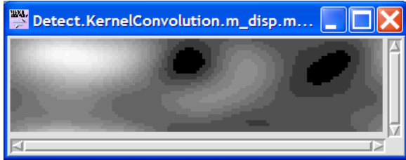
Figure 8 - This is the sound map after filtering and conversion to polar coordinates.
